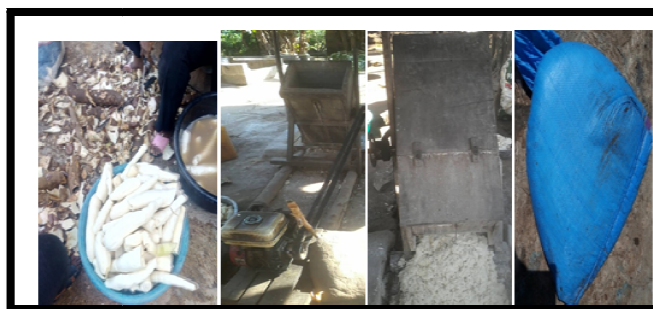
Figure 6: Peeled and Washed Cassava for Fermentation, Cassava Grater and Powering Engine, Grater Grating Cassava Tubers, Grated Flour Packed in a Bag
