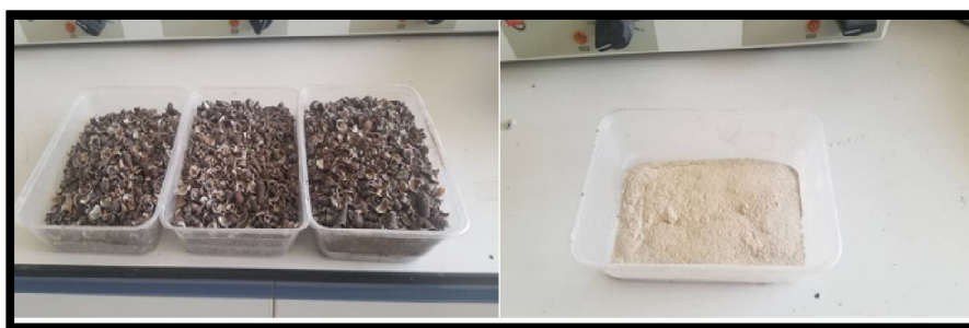
Figure 2: Periwinkle Shells Before and after Grinding
