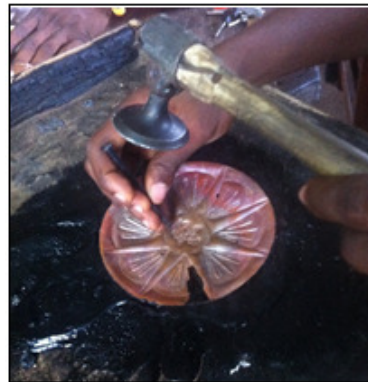
Figure 9: Chasing design on saucer
