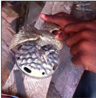
Figure 14: Filing cast piece
