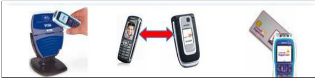
Figure 2: Examples of NFC Communication Modes
