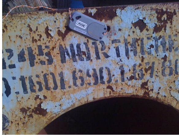
Figure 6: Tagging a Material Open Yard at NCTPS ( 2.4 GHz)
