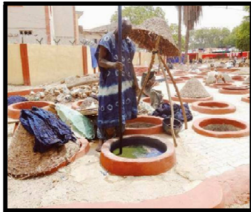
Figure 3: Showing the Mixture of Ash, Potassium, Chloride, the Indigo Plant and Lots of Water (Upto 1500 Litres) Is Pour into the Dyeing Pit and Left to Ferment before the Dyeing Commence
