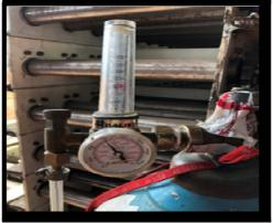
Figure 3: Shielding Gas Cylinder and Regulator
