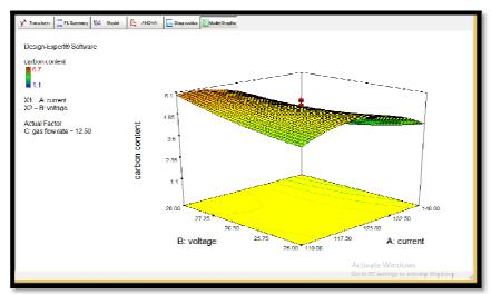
Figure 5: Effect Of Current and Voltage on Carbon Content
