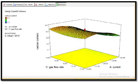
Figure 6: Effect of Current and Gas Flow Rate on Carbon Content
