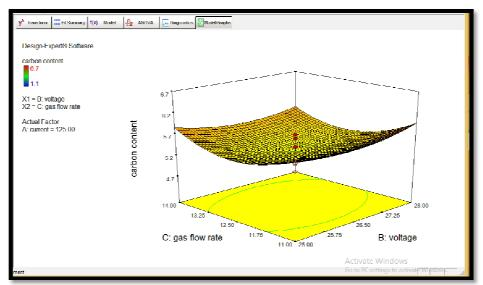
Figure 7: Effect of Voltage and Gas Flow Rate on Carbon Content
