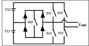
Figure 1: Fundamental cell of proposed MLI
