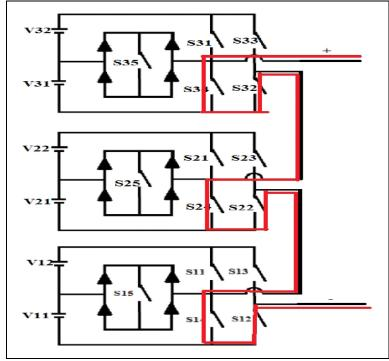
Figure 2: Proposed cascaded multilevel inverter
