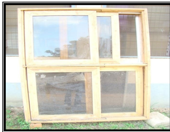
Figure 3: Window frame in bamboo (Preserved with dursban)
