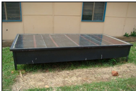
Figure 1b: The Black Body Radiative Trough For Preservative Treatment of Sympodial Bamboo Species in Ghana ( currently in use at the IRAI Dept KNUST.)
